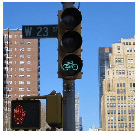
Intersection treatments such as two-stage turn queue boxes and bicycle signals allow bicyclists to cross high-traffic streets.
